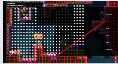
CelesteBot operating. Neural net is still early in training. Machine vision is represented by the white, green, and blue squares. White is air, green is solid tile, and blue is spike. Neural net is represented by red and green lines spanning input and output nodes.
